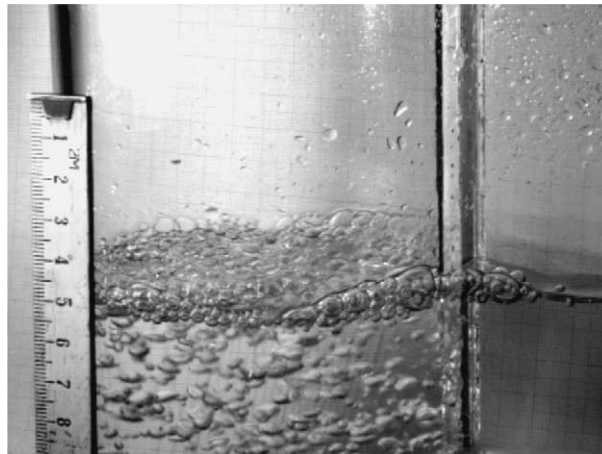
Fig. 9. Photograph of the water surface in the bubble column at a superficial velocity j_g = 0.195 cm/s; \epsilon = 0.012 .
